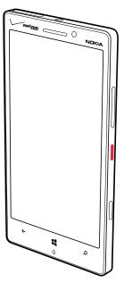
To turn the power off, press and hold the Power/Lock Key and then swipe your finger down the screen to shutdown.
