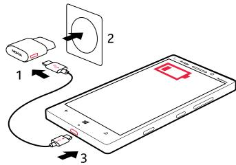
2. When the battery is full, disconnect the charger from the phone, then from the wall outlet.
