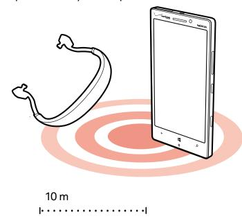
Since devices with Bluetooth wireless technology communicate using radio waves, they do not need to be in direct line-of-sight. Bluetooth devices must, however, be within 10 meters (33 feet) of each other, although the connection may be subject to interference from obstructions such as walls or from other electronic devices.
