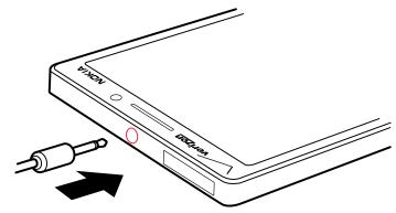
Do not connect products that create an output signal, as this may damage the device. Do not connect any voltage source to the Headset Connector. If you connect an external device or headset, other than those approved for use with this device, to the Headset Connector, pay special attention to volume levels.
