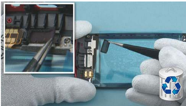
15) Use the tweezers to peel off the EARPIECE GASKET with MESH. Do not use it again.
