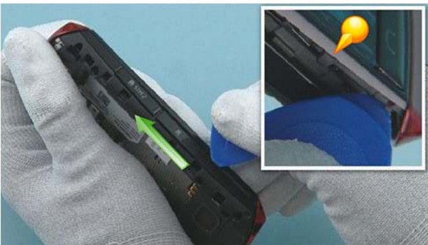
9) Release also the SIM DOOR side with the SRT-6.
