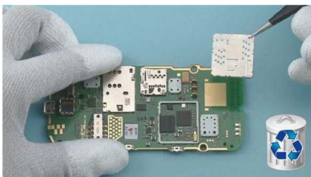
27) Remove the BB SHIELDING LID with the tweezers. Do not use the BB SHIELDING LID again. Discard it.
