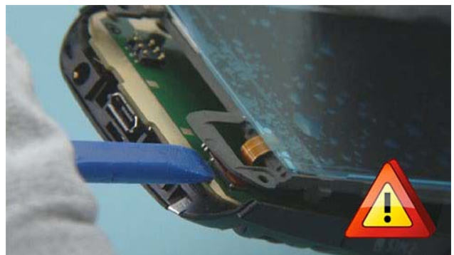
18) Disconnect the DISPLAY CONNECTOR with the SS-93. Be careful not to damage any components nearby.
