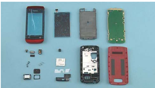
39) Now the Nokia Asha 305/306 disassembly procedure is complete.
