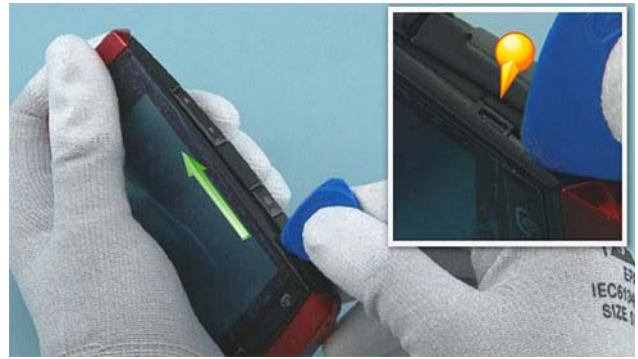
8) Continue to release the A-COVER with the SRT-6 on the VOLUME KEY side.
